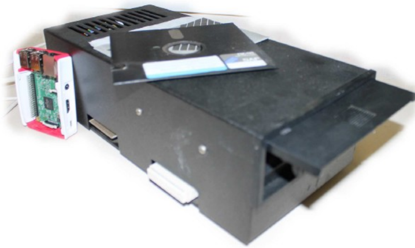
5.25" external floppy Drive for Video Genie & Raspberry Pi 3
